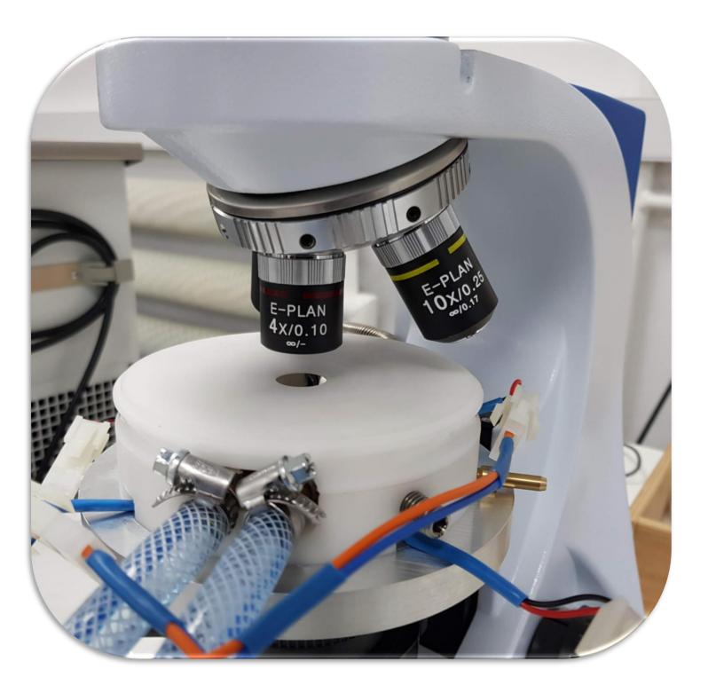
**Originally developed for microscopic observation of** phase transition of bio-materials at low temperature under European project SAFE ICE (2005).
